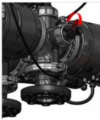
6. Open the command filter drain valve. In the On-line filter configuration, the drain is located at the bottom.
