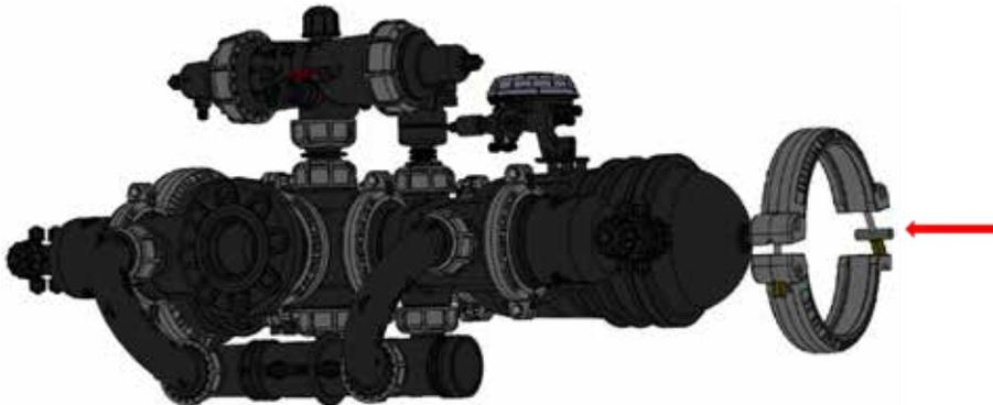
4. Keep pushing the cover while placing the upper clamp onto its location. Place the bottom clamp onto its location.
