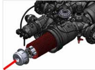
PLACE THE BUTTERFLY NUT ON TOP OF THE CYLINDER.
