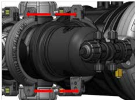
10. Remove the booster cylinder by pulling it backwards.
