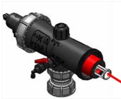
2. Close the command filter cover by tightening the cover nut.
