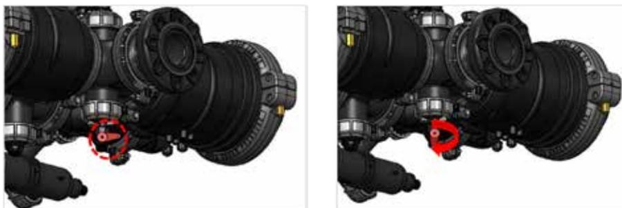
5. Open the command filter drain valve.
